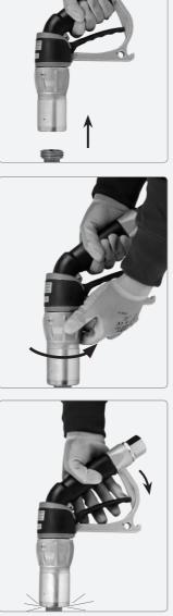
Deactivate lever latch (if fitted) by squeezing the lever
