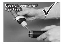
After connecting to the hose assembly, an operational test shall be performed. It is essential to examine that the nozzle, hose connector and swivel are tight under pressure and do not leak – e.g. by external application of foaming agents.
