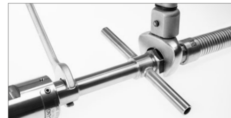
Connect the hose to the vent coupling. Torque to the hose fitting suppliers recommended tightening torque. Elaflex hose assemblies LNG 13: 60 Nm. Do not use pliers.
