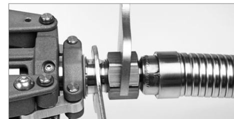
Connect the hose to the nozzle. Torque to the hose fitting suppliers recommended tightening torque of 150 Nm. Do not use pliers.
