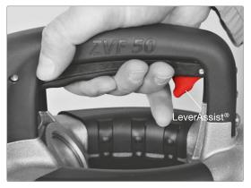
LeverAssist® reduces the necessary hold-open force of the lever by 75 %, making the fuelling process more comfortable. The 'Deadman' safety function' remains completely unaffected.
